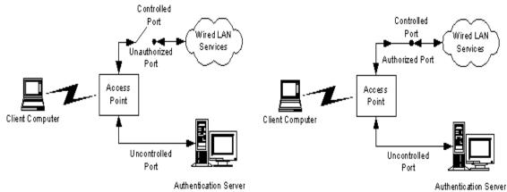
This diagram shows both the uncontrolled port used for authentication requests and the controlled port in its pre-authentication setting (left) and postauthentication setting (right.) As you can see, when a supplicant is successfully authenticated, the controlled port is considered authorized and communication through the logical port is allowed.
