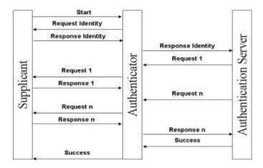
Please note that the first exchange of messages occurs between the supplicant and the authenticator, later exchanges occur between the supplicant and the authentication server without intervention from the authenticator.
