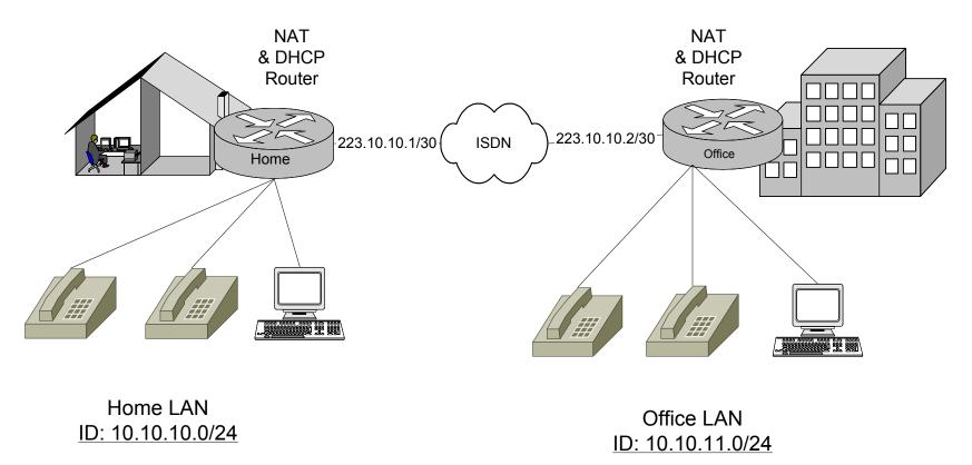
Configure an ISDN WAN connection (using legacy dial-on-demand routing) between the Home office and the HQ office which will be used to support voice and data communications between the two locations. Network Address Translations and Dynamic Host Configuration Protocol will be used at the two locations. Test your configuration by placing a call between the two locations and transferring files at the same time.
